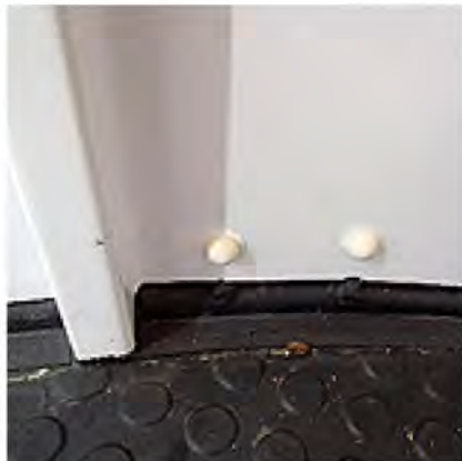
All rivets are rubber backed
