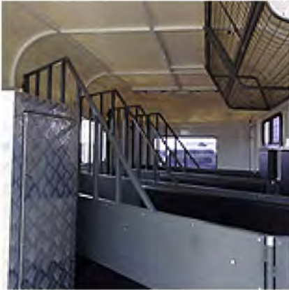
4 Horse float interior - saddle box, stalls & racks
