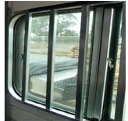
Horse float security window steel bars
