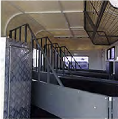
4 Horse float interior - saddle box, stalls & racks
